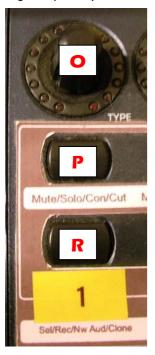
Picture to the left shows the controls at the top of a single track. Basic controls are as follows. O controls whatever the current rotary assignment is and can be activated by turning or pressing as appropriate for the current selection. Rotary assignment is covered in the previous sections.
